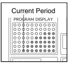
periods.) The speed setting for the first period will be shown in the flashing Current Period column of the matrix. The speed settings for the next seven periods will be shown in the columns to the right.
